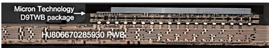
HMC package cross-section
