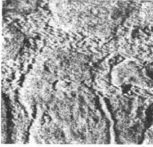
FIG. 8 Micrograph of etched brass produced by the SEM of Zworykin et al. (1942a); horizontal field width = 18 \mu\text{m} .
