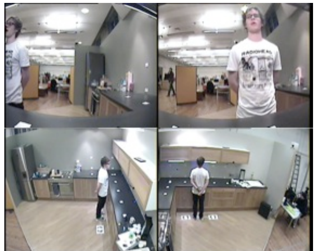
Figure 6. Simultaneously captured data from the embedded cameras allows us to develop a benchmark for attention detection algorithms based on tracking head pose and position from multiple viewpoints.
