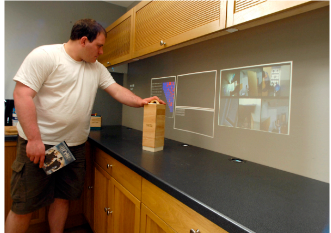
Figure 3. Using an RFID tagged control object the state of all the Ambient Kitchen sensors can be examined on the main display: floor pressure map (left); accelerometers (center-top); RFID (center-bottom); and video feeds (right).
