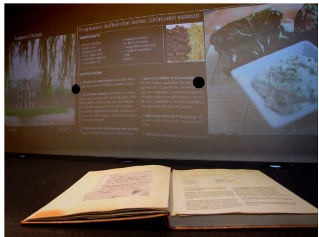
Figure 4. A current design scenario in which the pages of a cookbook have integrated RFID tags. The workbench can detect the current page and adapts the ambient display according to the page’s contents.
