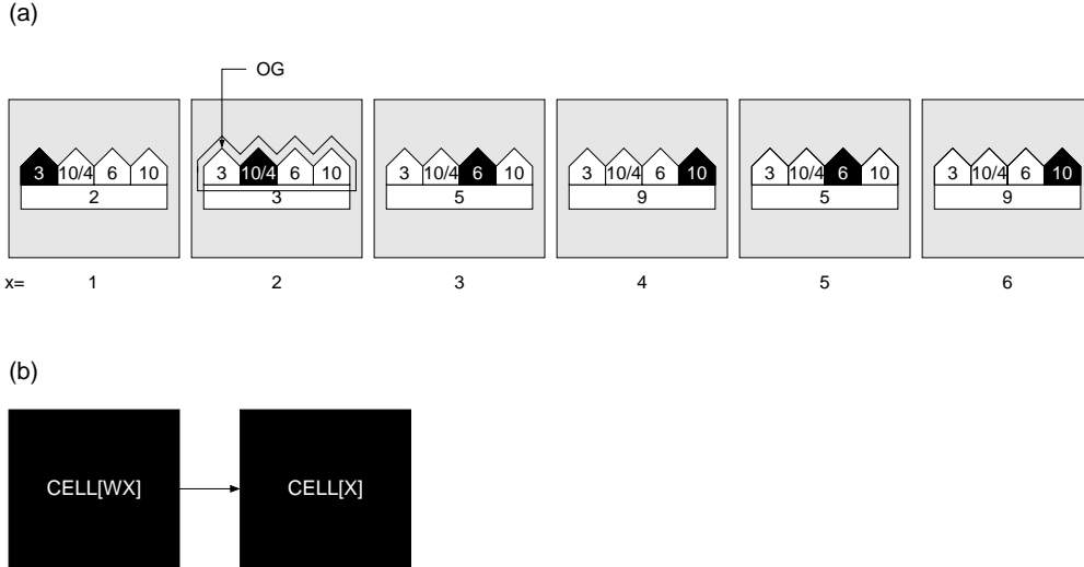
Fig. 3. Cellular differentiation of the BioWatch organism with operative genome and coordinates. (a) Global organization; OP: operative genome (genes and coordinates). (b) Central cell CELL[X] with its west neighbor CELL[WX] .
