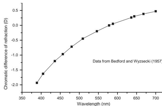
Fig. 8. Longitudinal chromatic aberration of the eye. Data from Wysecki and Stiles (1982) Table 1 (2.4.3) (originally reported by Bedford and Wysecki, 1957).
