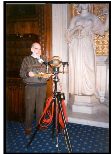
Recording in the Houses of Parliament with a 'dummy head' made from a converted outdoor light fitting
