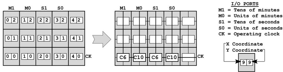
**Figure 5. Example of a coordinate-based system that places four cells of two different types (C6 and C10) in a 5x3 array according to a predetermined differentiation pattern to implement a timer.**
