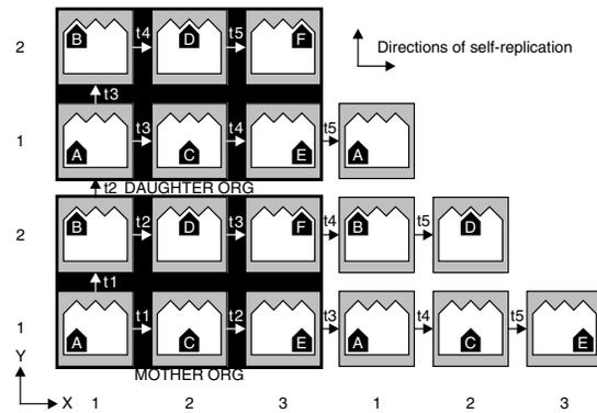
**Figure 3. Self-replication of a 6-cell organism in a limited homogeneous array. Only the expressed gene is shown in each cell.**
