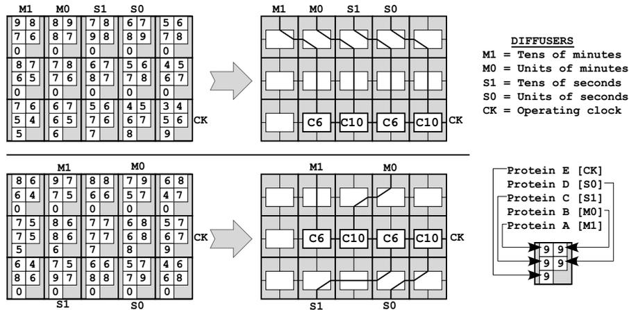
**Figure 6. Example of a gradient-based system that places four cells of two different types (C6 and C10) in a 5x3 array according to an environment-directed differentiation pattern to implement a timer. Depending on the position of the diffusers (I/O ports), the position of the cells changes.**
