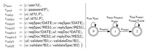
Fig. 4. Adaptation contract for our example: vectors (left) and VLTS (right).
