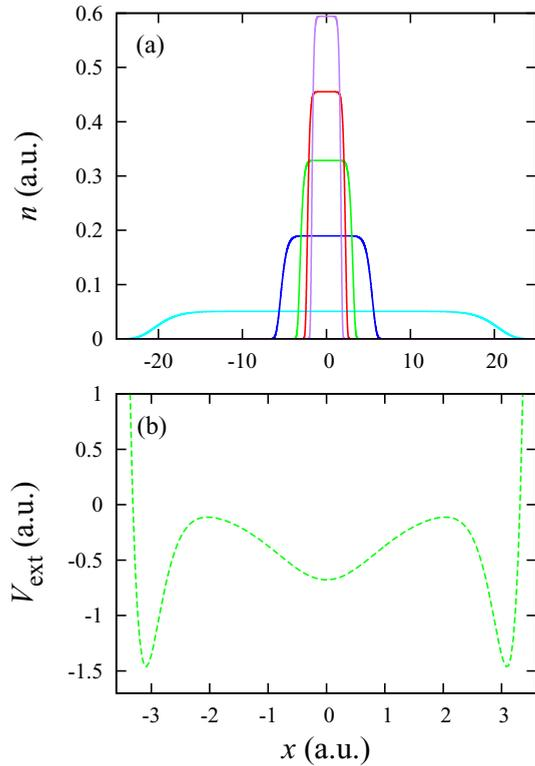
FIG. 1. (a) The exact many-body electron density (solid lines) for a selection of the two-electron slab systems. The density is of the form  $n(x) = n_0 \exp[-10^{-11}(mx)^{12}]$ , to generate a uniform plateau region that decays exponentially at the edges. (b) The optimized external potential (dashed green line) for a typical two-electron slab system [middle density in (a),  $n_0 \approx 0.33$ ].
