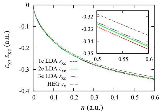
FIG. 4. The exact exchange energy  $\varepsilon_x$  (dotted-dashed dark-gray line) of a 1D HEG of density  $n$ . The  $\varepsilon_{xc}$  curves in the 1e (dashed red line), 2e (solid green line), and 3e (dotted blue line) LDAs are repeated from Fig. 3 for comparison. Inset: Close-up of the four curves at higher densities. All four curves are remarkably similar, indicating the importance of exchange in 1D, and showing the similarity of the different LDA approaches in 1D systems.
