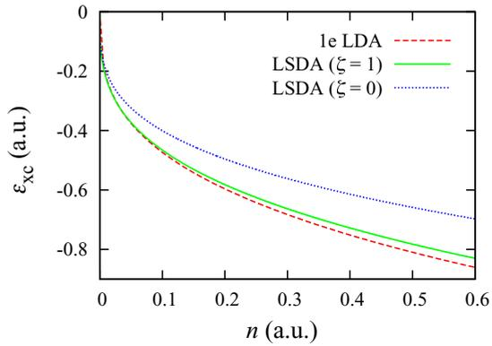
FIG. 5. The  $\varepsilon_{xc}$  curve (dashed red line) for the LDA that has been developed from 3D  $1e$  finite systems (which are fully spin-polarized), along with the fully spin-polarized ( $\zeta = 1$ ) (solid green line) and fully spin-unpolarized ( $\zeta = 0$ ) (dotted blue line) traditional LSDA [6]. We find the  $1e$  LDA and LSDA ( $\zeta = 1$ ) to be remarkably similar.
