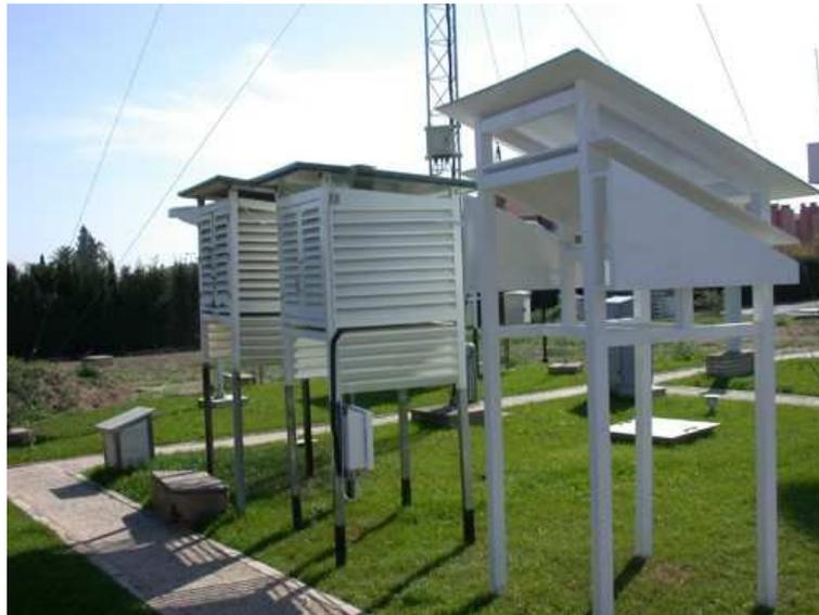
Figure 2.1: Different temperature observation equipment. Picture: Project SCREEN, Center for Climate Change, Universitat Rovira i Virgili, Spain. (CC BY 3.0)
