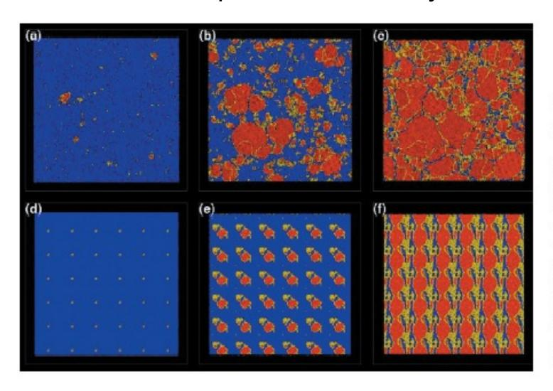
Snapshots from simulations of solidification in tantalum. The top sequence displays nucleation (a) and growth (b) occurring in a 16,372,000-atom simulation, resulting in a realistic distribution of grains and grain boundaries (c). The same process modeled using 64,000 atoms (d–f) produced the artificial final structure shown in (f).
