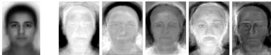
Figure 4-8 - Average face image and the first 5 eigenfaces defining a face space with no image pre-processing.
