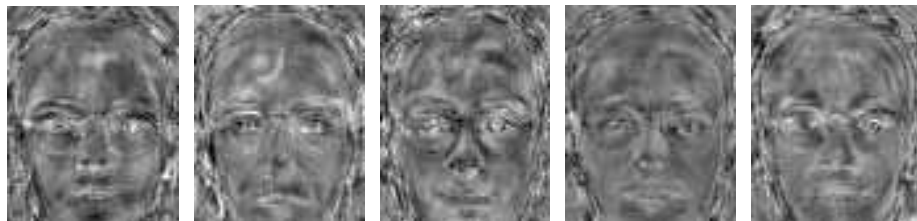
Figure 4-17 - The first five Fisherfaces, defining a face space with no image pre-processing
