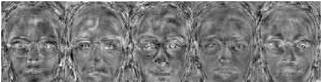
Figure 7-2 The first five Fisherfaces, defining a face space with no image pre-processing.
