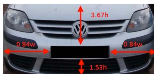
Figure 2. Example of an extracted region of interest, h is the license plate height and w is the license plate width.
