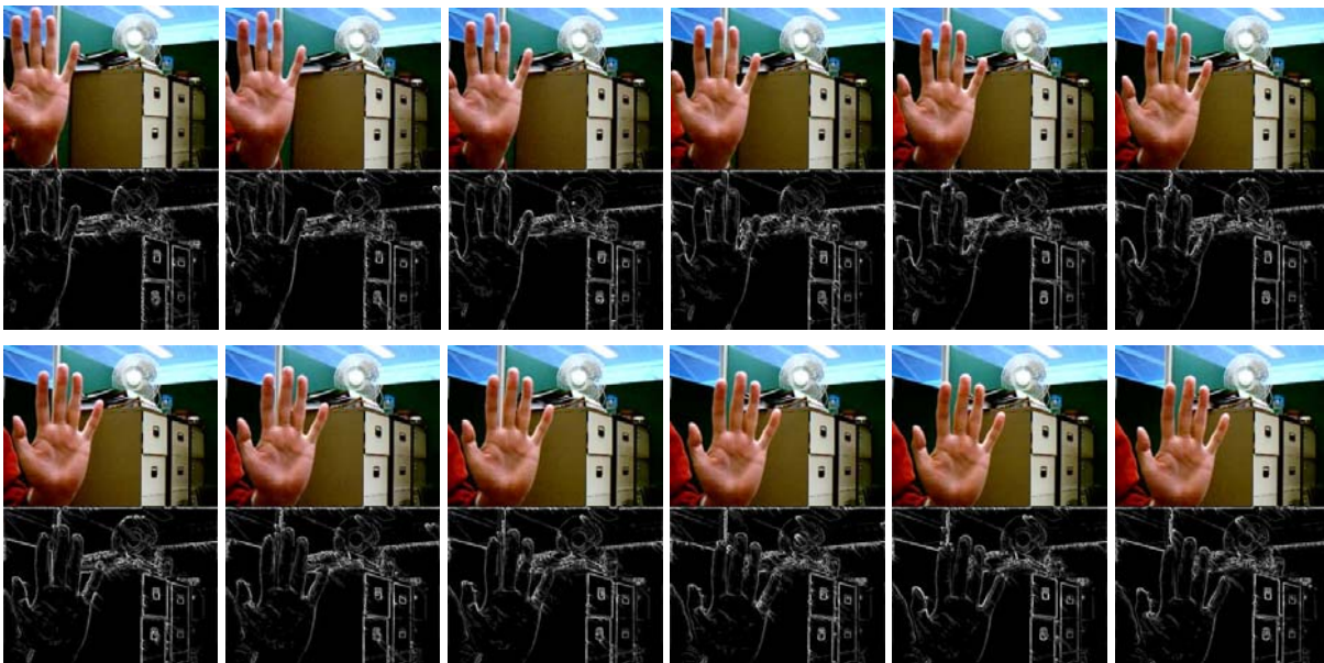
Figure 4: Screen shot of real-time video edge extraction with successive 12 frames in which the camera was fixed and the hand was moving.
