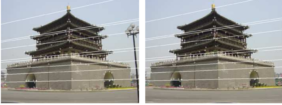
Fig. 1. A pair of images from the Xi'an Bell Tower sequence, showing 200 interest points (extracted using KLT) and some of the epipolar lines (computed using RANSAC).
