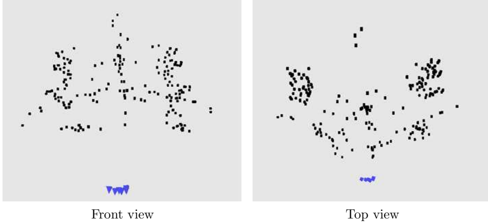
Fig. 2. Metric 3D model of sparse matched points and the positions of the camera.
