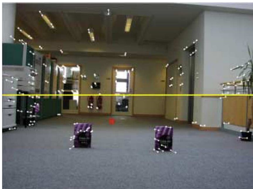
Fig. 10. Some correspondences, moving tracks (small line segment), the vanishing line and the FOE ( \circ ).
