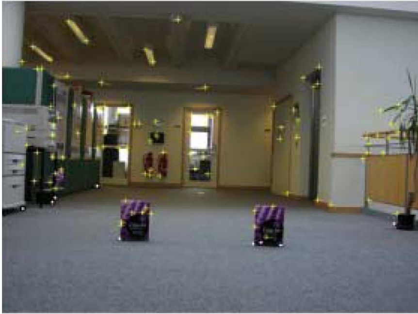
Fig. 11. The segmented coplanar points (·) and non-coplanar points (+).
