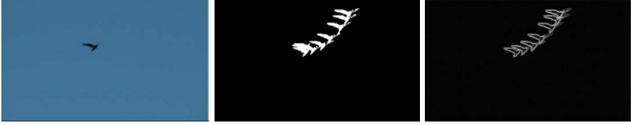
Fig. 2. In this video sample, a bird flies in the sky (left). The features MHI (middle) and MMHI (right) both have retained the motion information of the bird.
