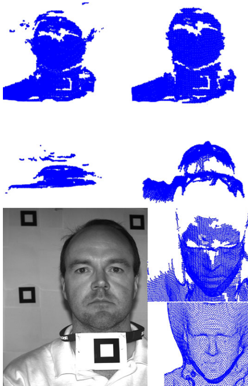
Fig. 11 The filtering process. Left column shows raw UoY data ( top and middle left are 3D, bottom left is 2D). Right column shows filtered 3D data and an RBF interpolated face ( bottom-right ), generated from a ‘marching cubes’ style algorithm. This is for illustration purposes: we do not need to compute this interpolated surface in order to generate our SSR descriptors, which are highly immune to missing parts in the raw data
