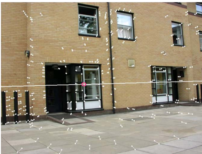
Fig. 9. One of the image pair with their matching points (●), displacement of feature points, FOE (o) and vanishing line.
