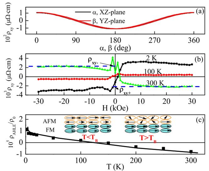
FIG. 3. (Color online) For IrMn/YIG, (a) the angular dependent  $\rho_{xy}$  in the  $xz$  (black line) and  $yz$  (red line) planes at 5 K and  $H = 10$  kOe, (b) the AHLE loops at  $T = 2, 100$ , and 300 K, and (c) the AHLE angle  $\rho_{\text{AHLE}}/\rho_0$  vs  $T$ . The insets in (c) schematically show the IrMn spin structure below and above  $T_B$ .
