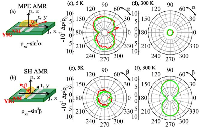
FIG. 1. (Color online) Measurement geometries of (a) the MPE AMR and (b) the SH AMR. In (a) and (b), the sensing electric current is applied along the  $x$  axis. Angular dependent  $\Delta\rho/\rho_0$  in (c), (d) the  $xz$  and (e), (f)  $yz$  planes at (c), (e) 5 K and (d), (f) 300 K for IrMn/YIG. Here, the red and green lines refer to the clockwise and counterclockwise rotations of the external magnetic field  $H = 10$  kOe, and  $\Delta\rho = \rho_{xx} - \rho_0$ .
