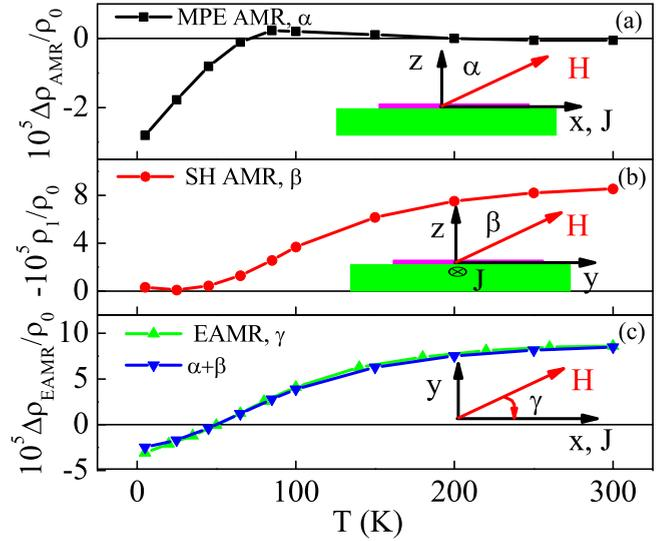
FIG. 2. (Color online) For IrMn/YIG, the  $T$  dependencies of (a)  $\Delta\rho_{\text{AMR}}/\rho_0$ , (b)  $-\rho_1/\rho_0$ , and (c)  $\Delta\rho_{\text{EAMR}}/\rho_0$ . The data in (a)–(c) were achieved from measurements of angular dependence in the  $xz$ ,  $yz$ , and  $xy$  planes under  $H = 10$  kOe, respectively. In (c), the sum of  $-\rho_1/\rho_0$  and  $\Delta\rho_{\text{AMR}}/\rho_0$  is also given.
