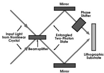
In the technique, two initially entangled photons, incident on opposite sides of a beamsplitter, would be routed to two grazing incidence mirrors. One of the paths would lead directly to a target, while the other would include a phase shifter before the target.
