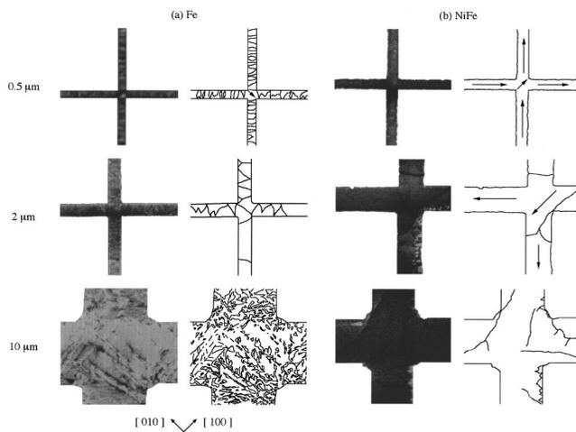
FIG. 3. MFM images and schematic diagrams of the domain configurations of the mesoscopic crosses (30 nm thick,  $w$   $\mu\text{m}$  wide, and 200  $\mu\text{m}$  long) of both (a) Fe and (b) NiFe as grown (unmagnetized states).
