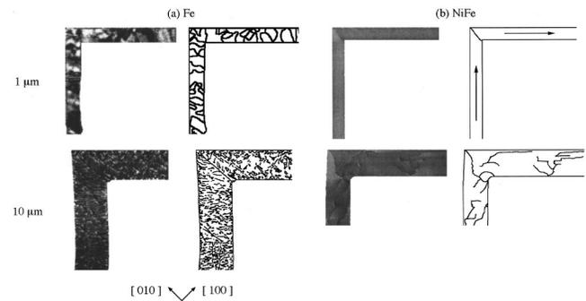
FIG. 2. MFM images and schematic diagrams of the domain configurations of the mesoscopic L shape structures (30 nm thick,  $w$   $\mu\text{m}$  wide and 200  $\mu\text{m}$  long) of both (a) Fe and (b) NiFe as grown (unmagnetized states).
