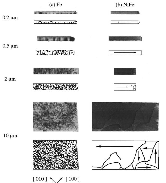
FIG. 1. MFM images and schematic diagrams of the domain configurations of the mesoscopic wires (30 nm thick,  $w$   $\mu\text{m}$  wide and 200  $\mu\text{m}$  long) of both (a) Fe and (b) NiFe as grown (unmagnetized states).
