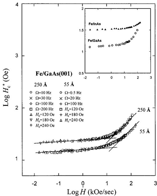
FIG. 1. Log–log plots of dynamic coercivity ( $H_c^*$ ) against field sweeping rate  $\dot{H}$  at various frequencies and field amplitudes for 55 and 250 Å Fe/GaAs(001) films. The lines are guides for the eye to distinguish two regions. The inset displays log–log plots of  $H_c^*$  against field sweep rate for the 250 Å Fe/GaAs(001) and 150 Å Fe/InAs(001) films.
