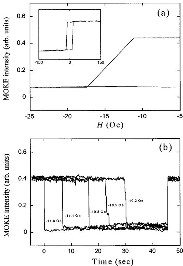
FIG. 3. Magnetic relaxation curves of 55 Å Fe/GaAs(001) film under a constant reverse field.
