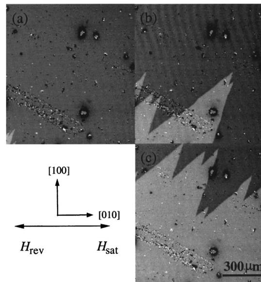
FIG. 4. Field-dependent evolution of domain structure at various fields in the 250 Å Fe/GaAs(001) film during the magnetization reversal process: (a) 24, (b) 29, and (c) 32 Oe.
