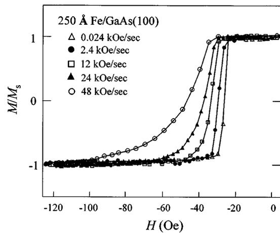
FIG. 2. Hysteresis loops of 250 Å Fe/GaAs(001) film in a negative magnetic field for several field sweep rates  $\dot{H}$ .
