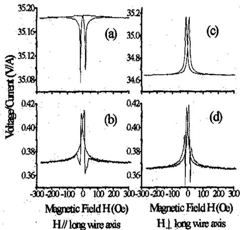
Fig. 2. (a), (c) AMR response curves ( $V_{23}/I$ ) and (b), (d) PHE response curves ( $V_{35}/I$ ) for the field applied parallel and perpendicular to the long axis of the device, respectively. In  $V_{ij}$ , the voltage is measured between terminals  $i$  and  $j$  when current flows from terminal 1 to terminal 4.
