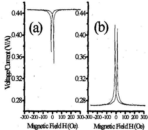
Fig. 3. PHE response curves with fields applied at (a)  $45^\circ$  (b)  $135^\circ$  with respect to the long wire axis of the device. The voltage is measured between terminals 3 and 5 when current flows from terminal 1 to terminal 4.
