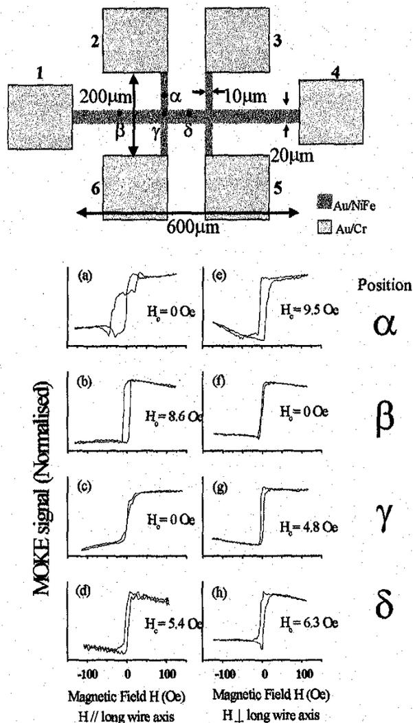
Fig. 1. Device geometry and microscopic MOKE hysteresis loops measured in four different positions ( $\alpha$ ,  $\beta$ ,  $\gamma$  and  $\delta$ ) of the device by scanning Kerr microscopy with the field applied parallel and perpendicular to the long axis of the device.
