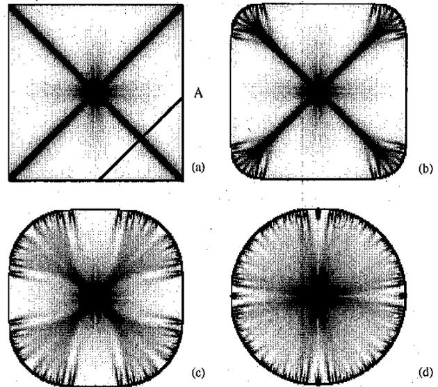
Fig. 3. Micromagnetic simulations for (a) a permalloy square ( $w = 5 \mu\text{m}$ ) and (d) a circular disk ( $r = 5 \mu\text{m}$ ) together with several intermediate states: a square with rounded corners  $r_c =$  (b) 0.9  $\mu\text{m}$  and (c) 1.8  $\mu\text{m}$ . Black lines connected with the corners correspond to magnetic domain walls.
