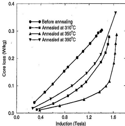
Fig. 1. Comparison of the effects of annealing temperature on core loss. Optimum reduction in core loss is obtained at around 350°C. Core-loss measurements were carried out at 1 kHz.
