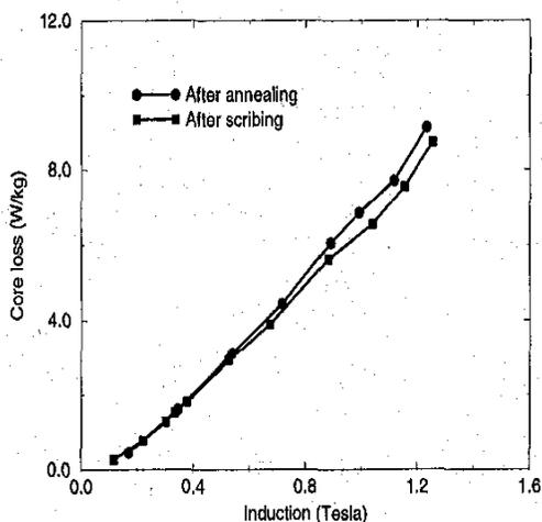
Fig. 4. Effects of continuous-wave laser scribing on core loss. Measurements were carried out at 1 kHz.
