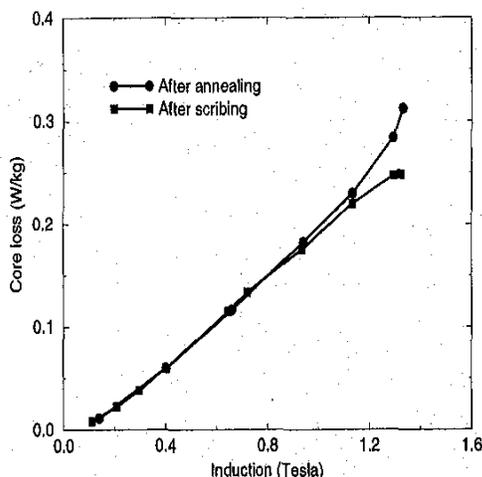
Fig. 3. Effect of continuous-wave laser scribing on core loss. Measurements were carried out at 50 Hz.
