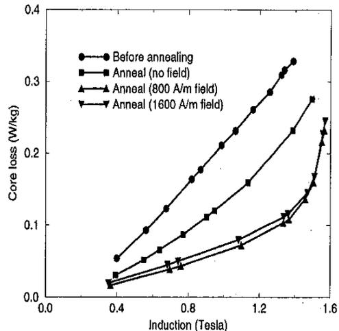
Fig. 2. The effects of a longitudinal field during annealing. A field of around 800 A/m was found to give the best results.
