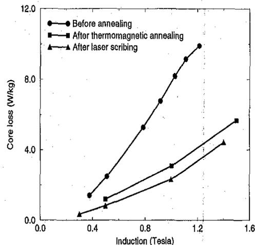
Fig. 5. Core-loss measurements at 1 kHz on the as-cast, magnetic-field annealed (350°C and 800 A/m) and laser surface scribed ribbons.
