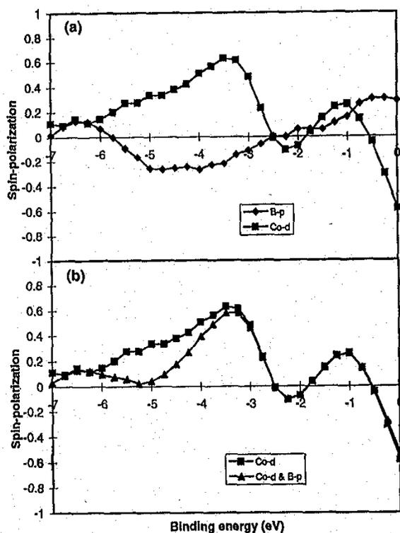
Fig.4. Variation with binding energy of the polarisation of *d* states of Co and *p* states of B estimated from Fig. 2 of [5]. (a) Shows the individual states while (b) is a comparison of the *d* states with a summation of the *d* and *p* components weighted by their *d* and *p* partial densities of states.
