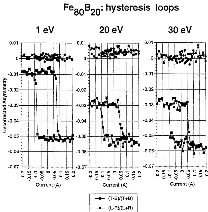
Fig. 3. The spin polarized detection system operated as a surface magnetometer: hysteresis loops for Fe<sub>80</sub>B<sub>20</sub> at secondary electron energies 1, 20 and 30 eV. The left and right detectors (L and R) show no asymmetry on average, while the top and bottom detectors follow the near surface magnetisation ( $\propto (T - B)/(T + B)$ ).
