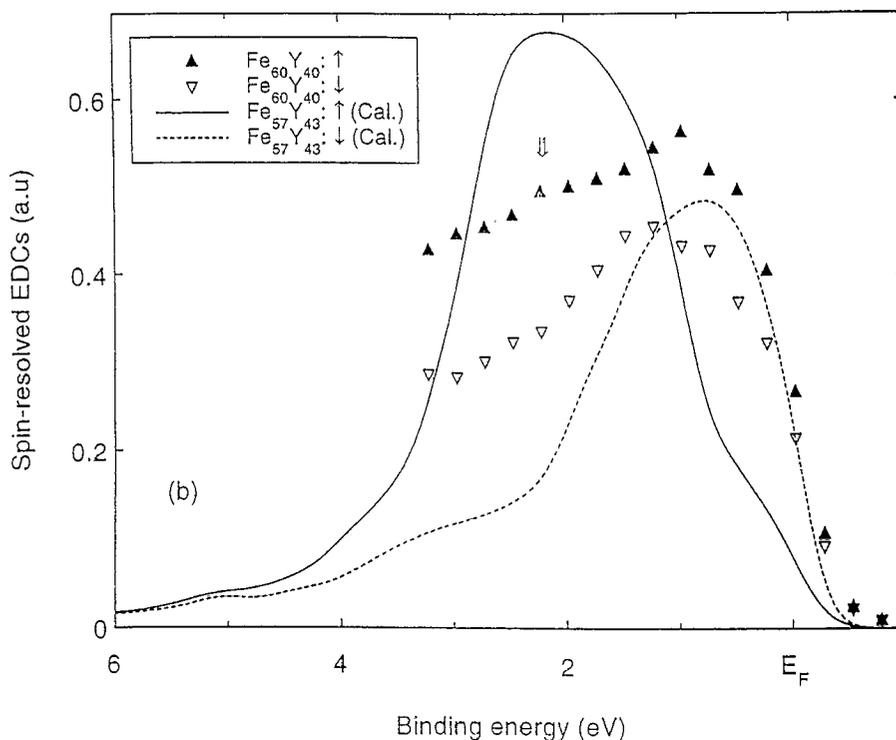
Fig. 5. Experimental spin resolved EDC curves of  $\text{Fe}_{60}\text{Y}_{40}$  [6] compared with theoretical spin resolved bulk densities of states of  $\text{Fe}_{57}\text{Y}_{43}$  of Becker and Hafner [3], broadened to take account of experimental energy resolution.
