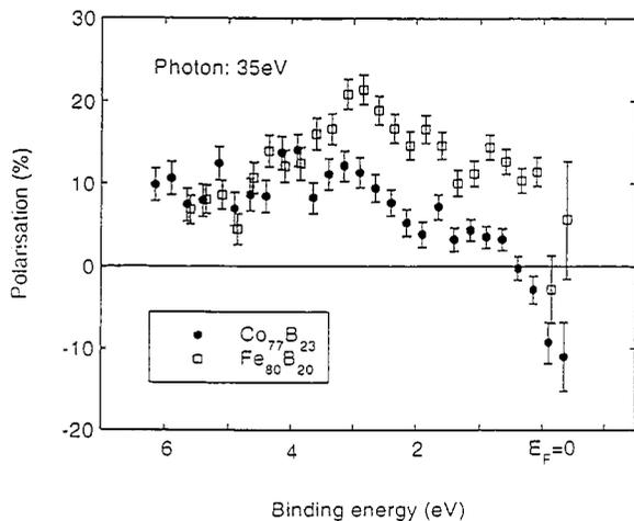
Fig. 2. Comparison of the spin polarization of  $\text{Fe}_{80}\text{B}_{20}$  and  $\text{Co}_{77}\text{B}_{23}$  for a photon energy  $h\nu = 35\text{ eV}$  [5].
