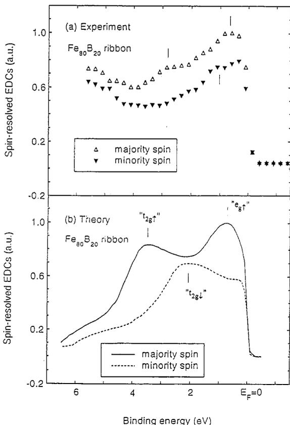
Fig. 4. (a) Experimental spin resolved electron energy distribution (EDC) curves of amorphous  $\text{Fe}_{80}\text{B}_{20}$  [5]. (b) Theoretical spin resolved bulk density of states by Hafner *et al.* [2], broadened to take account of the experimental energy resolution.
