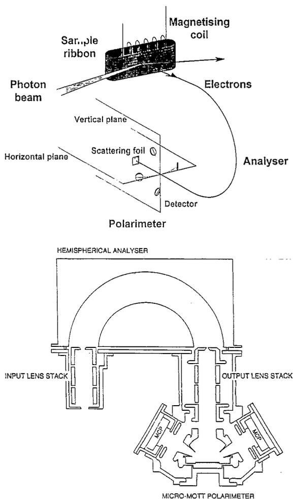
Fig. 1. Schematic diagram of the Daresbury spin detection system.
