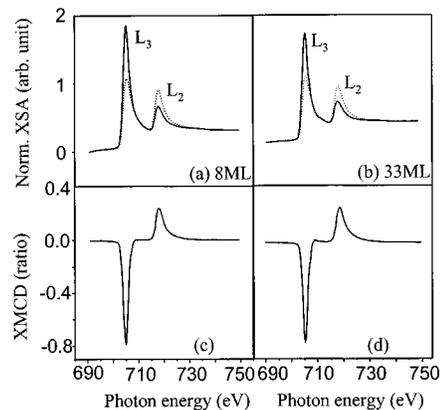
FIG. 1. (a) and (b) normalized XAS and (c) and (d) XMCD spectra of 8 and 33 ML films, respectively, with both the external magnetic field and the photon beam applied perpendicular to the film plane.
