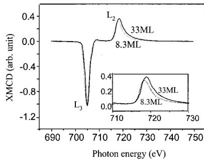
FIG. 2. XMCD spectra of the 8 and 33 ML films scaled to 1 at the peak of the  $L_3$  edge. The difference between the  $L_2$  peaks is shown clearly in the inset.
