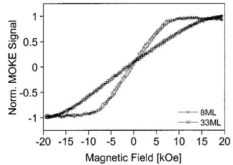
FIG. 3. Magnetization loops of the 8 and 33 ML films with the field applied perpendicular to the film plane measured with polar MOKE.
