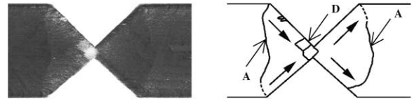
Fig. 2. MFM images of the permalloy bowtie (30 nm thick, 10 \mu\text{m} wide and 210 \mu\text{m} long) in the remanent state after the application of magnetic field along the wire.
