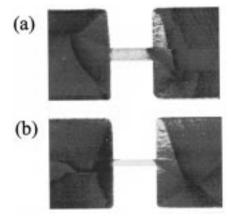
Fig. 4. MFM images of the bridge structure with (a)  $w = 1 \mu m$  and (b)  $w = 0.5 \mu m$  in the demagnetized state. The narrow regions with w = 0.5,  $1 \mu m$  show a single domain state, while multidomains are seen in the wide wires.
