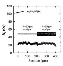
Fig. 1. The variation of the switching field as a function of position for the wire junction structure ( $w_1 = 1 \ \mu m$ ,  $w_2 = 5 \ \mu m$ ), measured every 10  $\mu m$  along the wire length. The arrow indicates  $H_c$  in the fixed width wire ( $w_1 = w_2 = 1 \ \mu m$ ) obtained by MR measurement.
