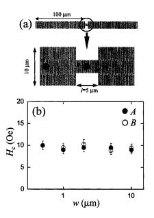
Fig. 3. (a) Schematics of the bridge structures, which have a narrow region with a length  $l = 5 \mu$  m and a width  $w = 0.5-10 \mu$ m introduced in the center of the wire. The dots on the schematics denote the fixed positions **A** (50  $\mu$ m away from the end of a wide wire) and **B** (center of the narrow wire) of the laser beam spots. (b) The variation in the switching field ( $H_c$ ) against the wire width of the narrow region.
