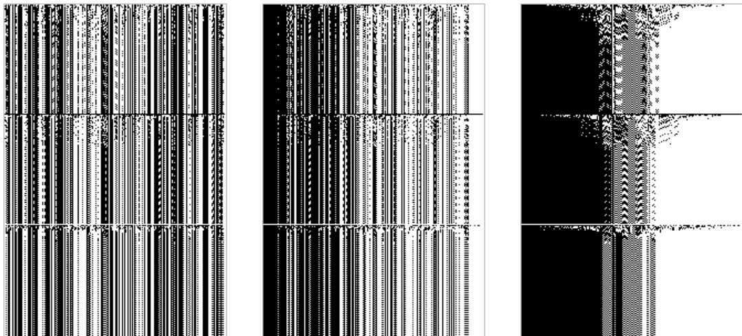
Figure 3.6 Visualisation of the time evolution of a typical K = 2 RBN, with N = 200 , and initial condition all nodes randomised (50% “on”, 50% “off”); reinitialised after 100 timesteps with all nodes “on”; reinitialised after a further 100 timesteps with all nodes “off”. (a) left: unsorted (as figure 3.3); (b) middle: sorted on boolean function value; (c) right: sorted on frozen core activity (as figure 3.4)
