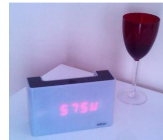
figure 1. The Wattson energy monitor from DIY Kyoto
