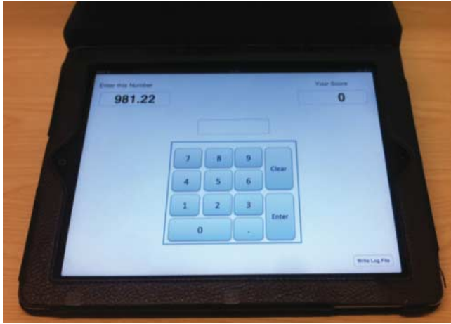
Figure 1. Experimental set-up: iPad running the number-entry app in the clear condition with the number to-be-transcribed in the upper left corner and the target area in the centre above the number-pad.
