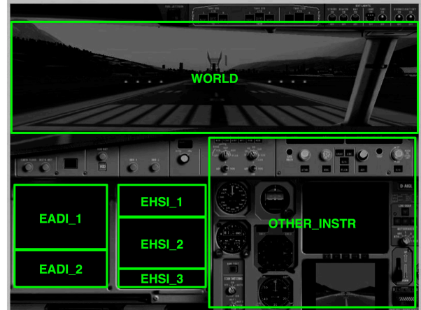
Figure 4. Definition of the AOIs on the cockpit of the Boeing 737-900ER.
