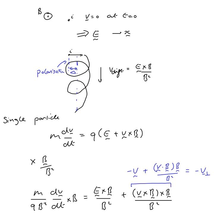
$$V_{\perp} = \frac{E \times n}{n^2} - \frac{m}{q n^2} \frac{d u}{d t} \times n$$
