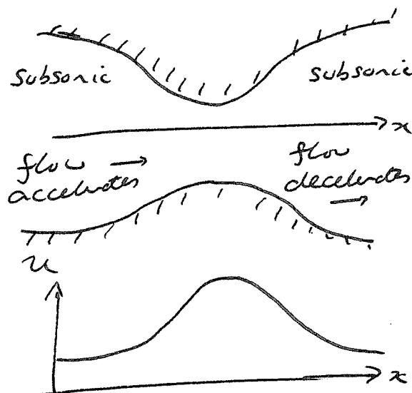
If the flow rate is too low then the fluid never reaches the local sound speed. As the nozzle expands, the flow slows down.
