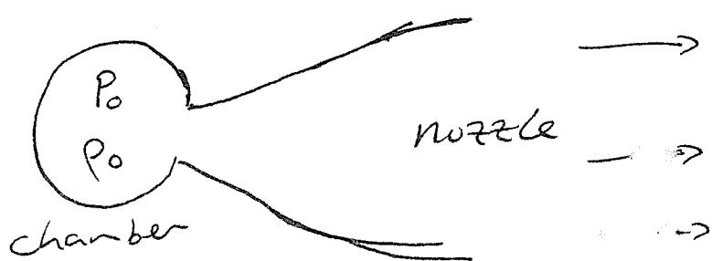
Fuel is burnt in a chamber sustaining a pressure  $P_0$  and density  $\rho_0$
