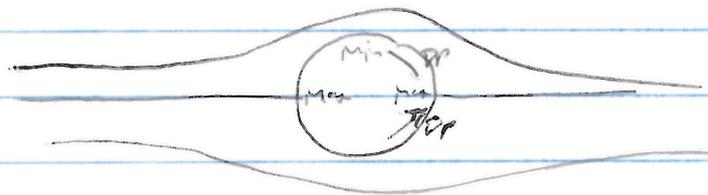
Increasing pressure in direction of flow can lead to separation of boundary - see later in course.
