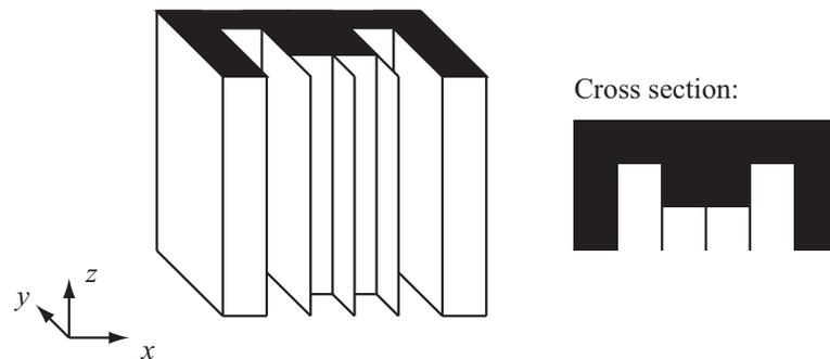
**Figure 5.3:** 3-D diagram of a simple Schroeder diffuser with cross section.
