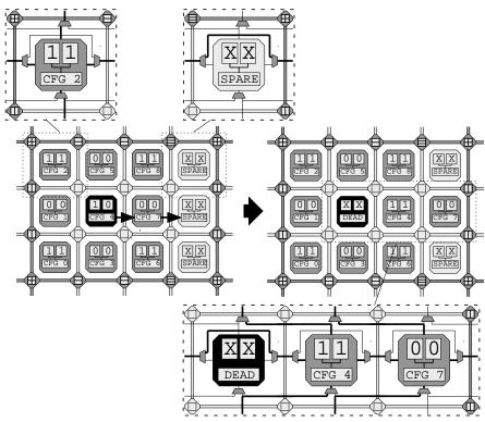
Figure 5: A fault is detected and the array is reconfigured to avoid the faulty element.
