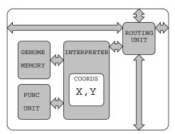
Figure 1: Structure of an electronic cell.
