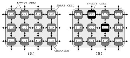
Figure 2: The electronic organism with no faults (A) and after reconfiguration (B).
