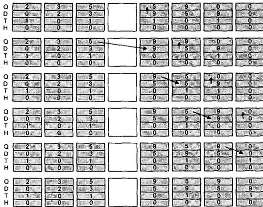
Figure 9. Time-preserving self-repair process of the BioWatch organism.
