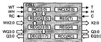
Figure 6. Block diagram of the BioWatch artificial cell.
