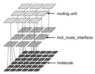
Figure 4. The tissue is actually composed of 3 layers: the molecules, the interface, and the routing units (not all connections are shown between molecules and interfaces).
