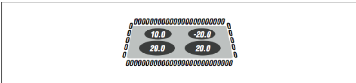
A two-dimensional plate with four constant heat sources
