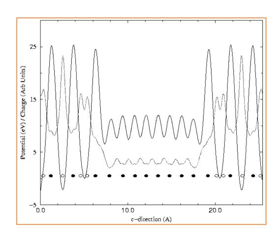
Offset is 0.4eV – useful for LED's and near-IR detectors
