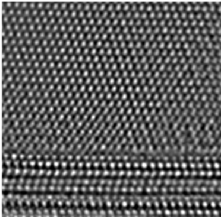
TEM of MgO(111) on SiC substrate
