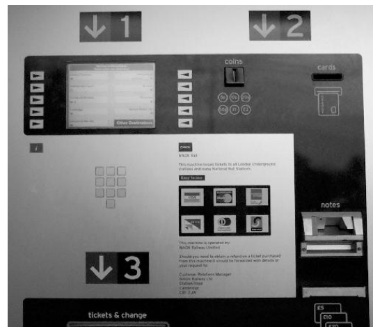
Figure 1: The ticket vending machine. The screen (diagonal 25cm, underneath the ‘↓ 1’ arrow) is at eye level for a standing adult, its centre 1.47m off the ground. There are five hard buttons on each side of the display screen (looking like triangular arrows) with meanings as displayed on the screen. There are two buttons with fixed meanings, for information (blue, on the left) and for cancelling (red, on the right). There are ten unlabelled buttons beneath the display that do nothing. The user can insert coins, credit cards or paper currency (underneath the ‘↓ 2’ arrow). A slot at the lower right, that looks like it might accept proprietary tokens, is apparently used as an alternative slot to return rejected notes. Tickets and change are obtained at the bottom of the machine, under the ‘↓ 3’ arrow.
