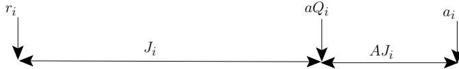
Figure 3. The time line of message \mu_i from its initiating event until it is able to participate in bus arbitration.
