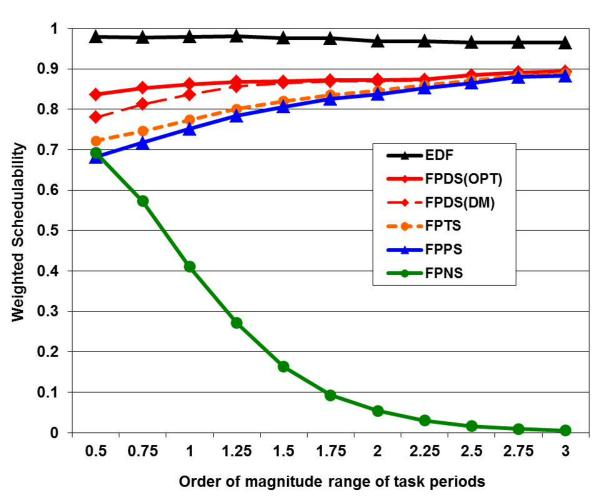
Constrained deadlines Taskset cardinality n = 10Variable range of periods Deadlines in the range  $[C_i + \alpha(T_i - C_i), T_i]$
