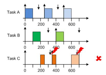
For FPPS deadline monotonic is the optimal priority assignment
