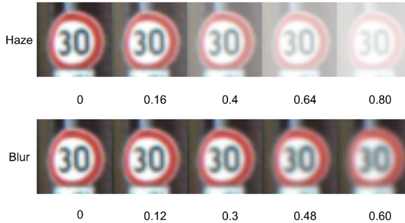
Fig. 3: Perturbed samples from the GTSRB dataset showing the independent effects of the influencing factors. Numbers under the images indicate the level of the effect applied.
