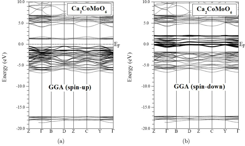
Fig. 4. The calculated spin-polarized band structures (a) spin up and (b) spin down at the equilibrium lattice constant of the monoclinic double perovskite  $\text{Ca}_2\text{CoMoO}_6$  compound using GGA-PBE. The horizontal dashed line indicates the Fermi level.
