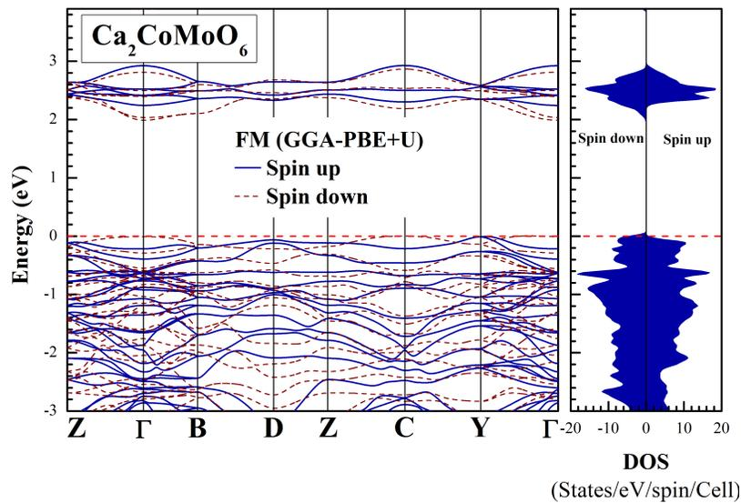
Fig. 7. The calculated spin-polarized band structure and total DOS of the monoclinic double perovskite  $\text{Ca}_2\text{CoMoO}_6$  compound in the FM configuration using GGA-PBE+ $U$ . The vertical dashed line indicates the Fermi level. The positive and negative values of DOS represent the spin-up and spin-down states, respectively.
