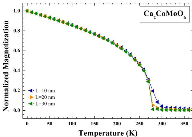
Fig. 8. The temperature dependent magnetization of the monoclinic double perovskite  $\text{Ca}_2\text{CoMoO}_6$  compound calculated using the atomistic spin model implemented in the Vampire software package.<sup>17,18</sup>
