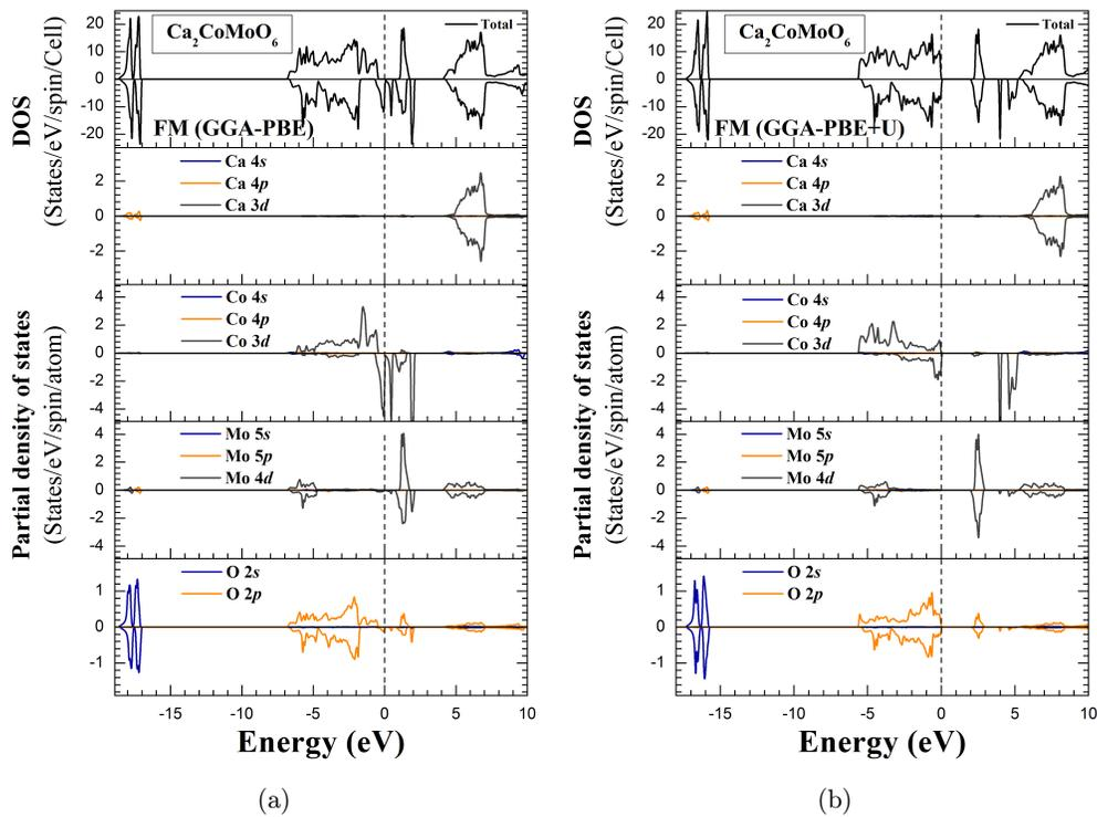
Fig. 6. The calculated spin-polarized total and partial DOS of the monoclinic double perovskite  $\text{Ca}_2\text{CoMoO}_6$  compound using (a) GGA-PBE and (b) GGA-PBE+ $U$ . The vertical dashed line indicates the Fermi level. The positive and negative values of DOS represent the spin-up and spin-down states, respectively.
