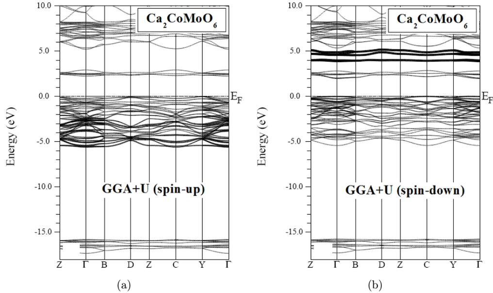
Fig. 5. The calculated spin-polarized band structures (a) spin up and (b) spin down at the equilibrium lattice constant of the monoclinic double perovskite  $\text{Ca}_2\text{CoMoO}_6$  compound using GGA-PBE+ $U$ . The horizontal dashed line indicates the Fermi level.
