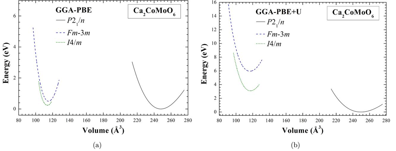
Fig. 1. Total energy as a function of volume for the ferromagnetic (FM) spin ordering of  $\text{Ca}_2\text{CoMoO}_6$  compound in the cubic, tetragonal, and monoclinic structures using (a) GGA-PBE and (b) GGA-PBE+ $U$ .
