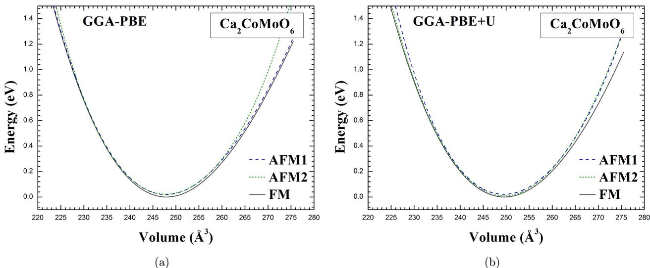
Fig. 3. Total energy as a function of volume for the ferromagnetic (FM) and anti-ferromagnetic [AFM1 and AFM2] spin orderings of the monoclinic  $\text{Ca}_2\text{CoMoO}_6$  compound using (a) GGA-PBE and (b) GGA-PBE+ $U$ .
