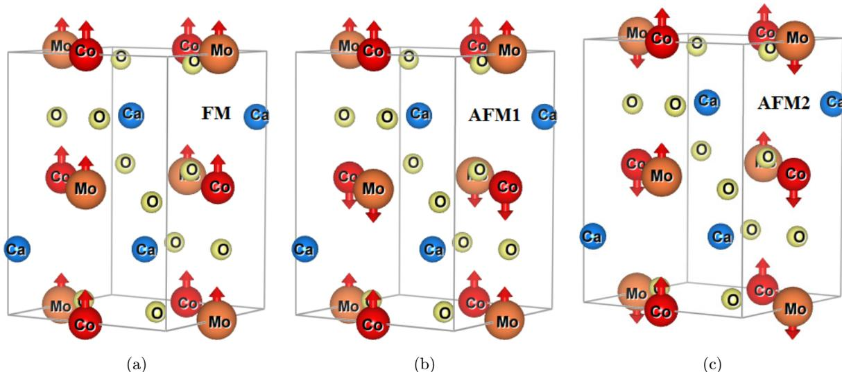
Fig. 2. Schematic representation of (a) ferromagnetic FM and the anti-ferromagnetic (b) AFM1, and (c) AFM2 spin configurations of  $\text{Ca}_2\text{CoMoO}_6$  crystal structure in the monoclinic phase produced by VESTA.<sup>20</sup>
